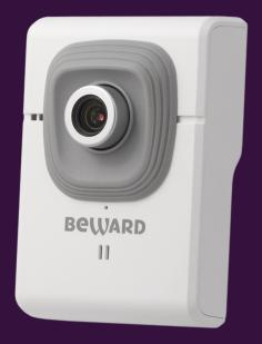
MicroSD/SDHC card slot Wi-Fi 802.11 b/g/n. WPS support 16 channel surveillance software included
