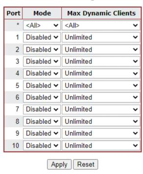
Figure 4-5-7-1: IP Source Guard Configuration Screen Page Screenshot
