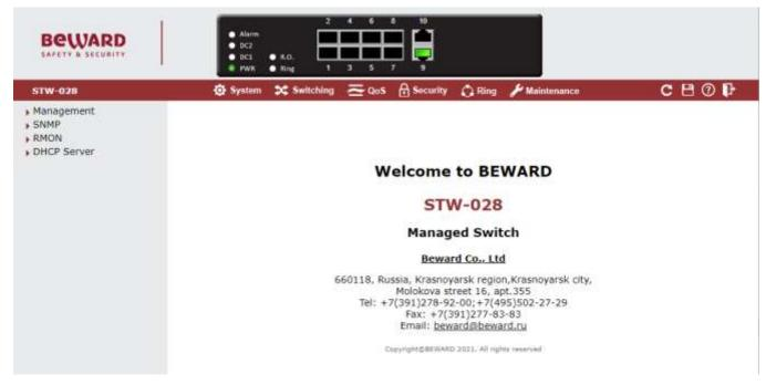
Figure 3-3: Web Main Screen of Managed Metro Switch
