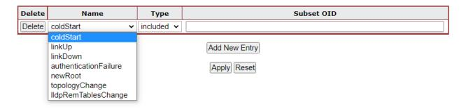
Figure 4-2-2-6: SNMP Trap Source Configuration Page Screenshot
