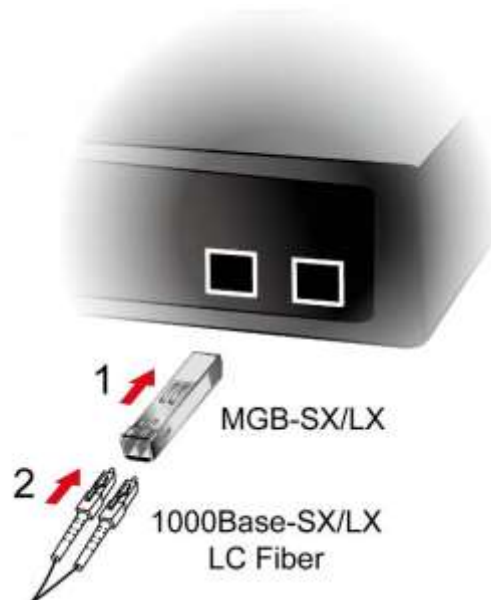
Figure 2-2-1 Plug in the SFP transceiver
