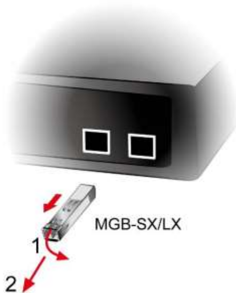
Figure 2-2-2 How to Pull Out the SFP Transceiver
